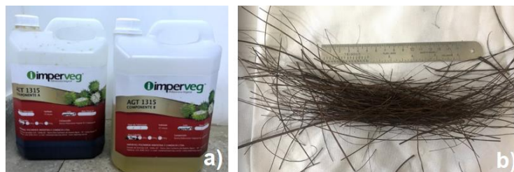
Figure 1. Castor oil based polyurethane resin (a) and the piassava Industrial waste fibers (b).
