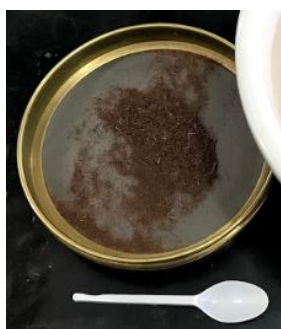
Figure 2. Piassava fiber particles after the shred process.
